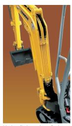
Hydraulic hose installed inside the boom bracket for damage prevention. Superb hydraulic piping distribution for clear front visibility.
